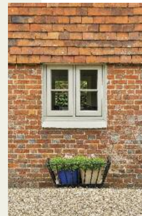
Flush casement windows finished in 'French Grey' externally and a colour complementary to Farrow & Ball 'Wimborne White' internally, with 18mm astragal glazing bars. Manufactured in Engineered Meranti Hardwood.
