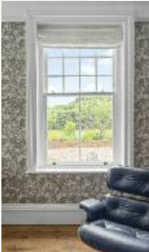
Slim sash windows finished in 'Off-White' with 18mm astragal glazing bars and decorative sash horns. Featuring Mottled Antique Brass hook fasteners, sash lifts and limit stop. Manufactured in Engineered European Redwood.
