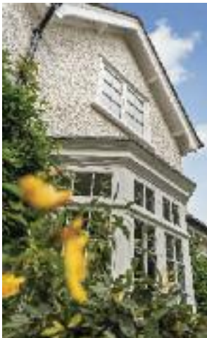
Flush casement windows finished in 'White' with 18mm astragal glazing bars and Polished Brass Peardrop handles and matching pegstays. Manufactured in Engineered European Redwood.
