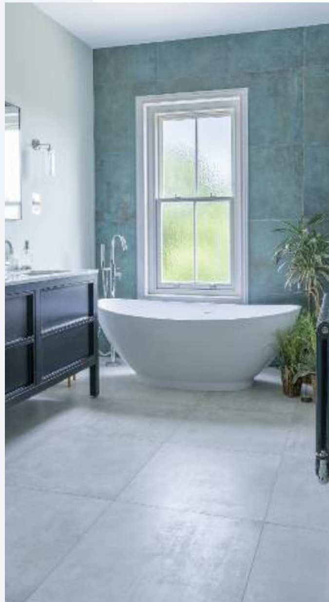
Slim sash windows with hidden spring mechanisms and 18mm astragal glazing bars, finished in “Off-White”. Manufactured in Engineered European Redwood.
