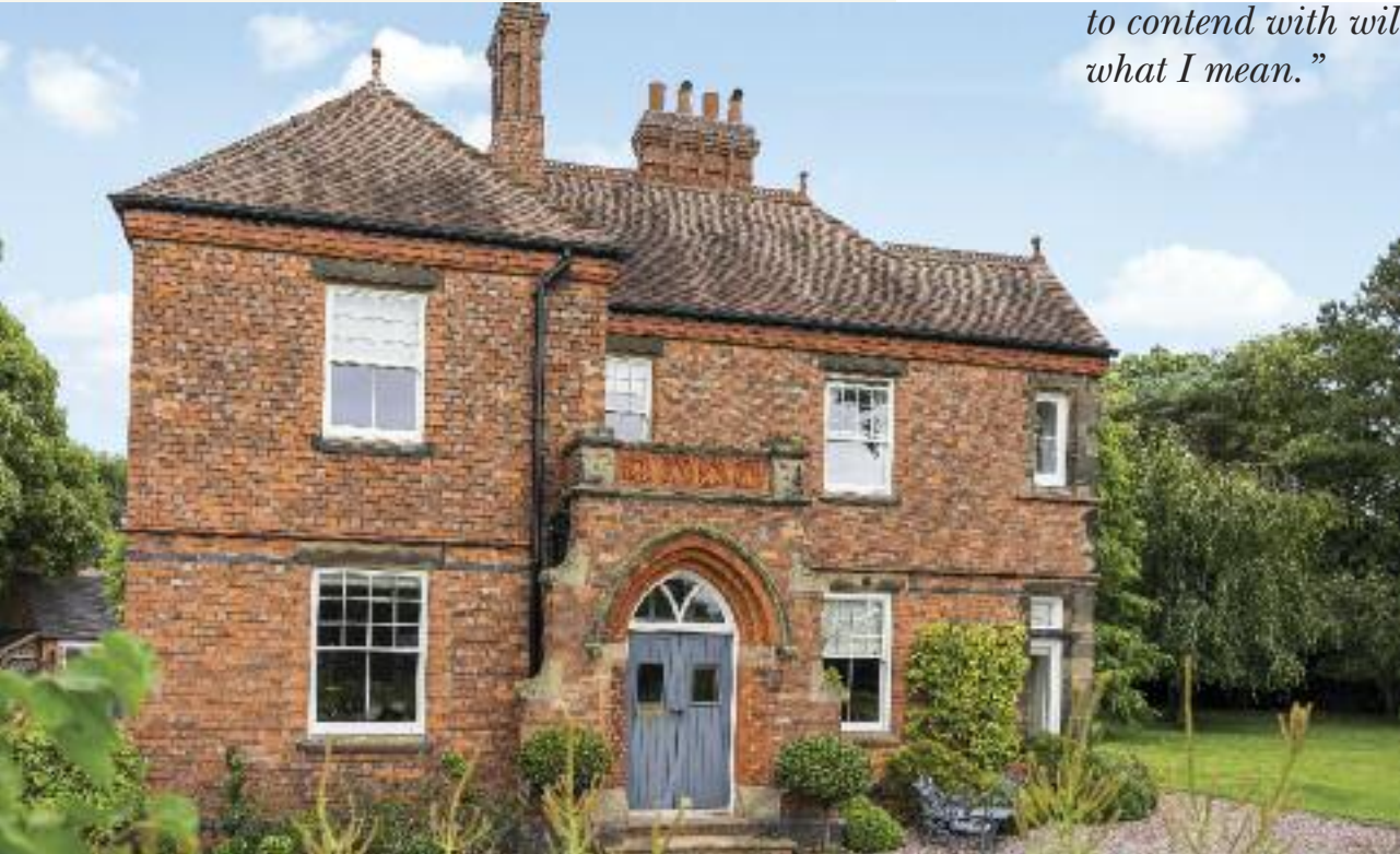
Slim sash windows finished in 'Off-White' with 18mm astragal glazing bars and decorative sash horns. Featuring Mottled Antique Brass hook fasteners, sash lifts and limit stop. Manufactured in Engineered European Redwood.
